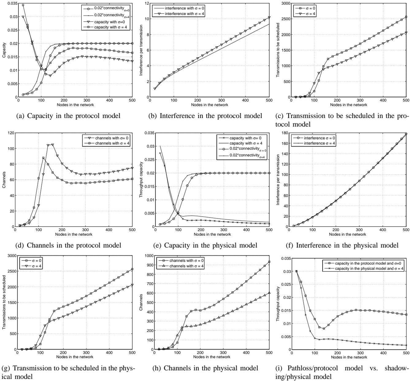
Fig. 5. Effects of log-normal shadowing radio propagation for both protocol and physical interference
