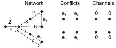
Fig. 1. Channel assignment under protocol interference. The straight line arrows represent the transmissions. The numbers assigned to the arrows refer to the distance the two corresponding nodes are apart. There is no conflict between any transmission and  $e_1$  since all other nodes are farther apart (Algorithm 1). Note that both conflict graph and channel assignment are considered as temporary snapshots from the perspective of  $e_1$ .
