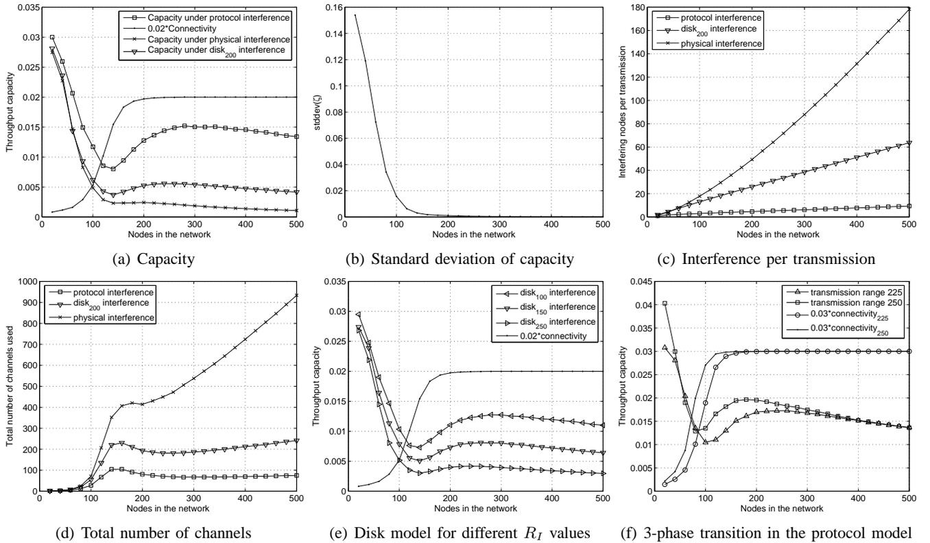
Fig. 4. Capacity under different interference models using path loss radio propagation
