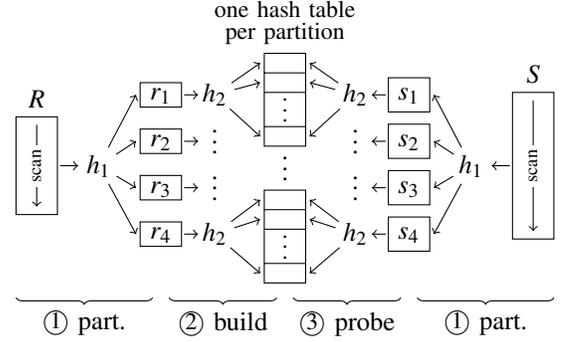
Fig. 3. Partitioned hash join (following Shatdal et al. [7]).
