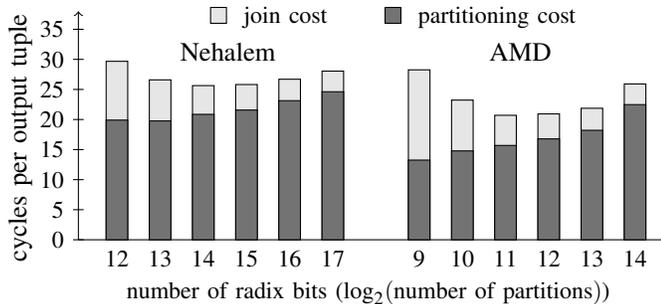
Fig. 9. Cost vs. radix bits (Workload **B**; Nehalem: 2-passes; AMD: 1-pass).
