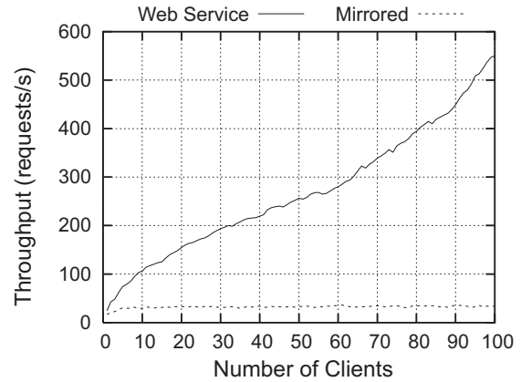
Fig. 3. Comparison of the throughput when calling a raw Web service and the create resource operation of the WS-Resource
