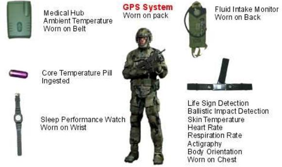
Figure 1: WPSM-IC Sensor System
