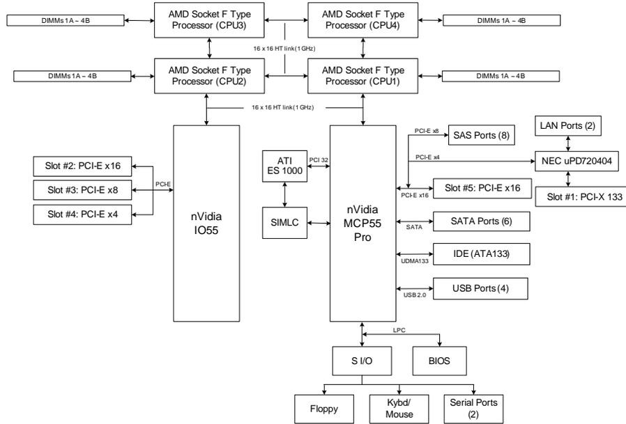
Figure 6: Block diagram of the mainboard.<sup>3</sup>
