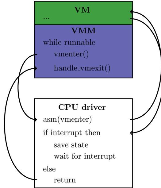
Figure 3: Non interrupted VMENTER/VMEXIT flow on one CPU.
