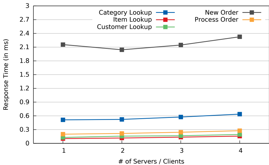
Figure 5.8: Scale-Out for 1 to 4 storage server / processing clients showing response times for individual queries when running the mixed workload
